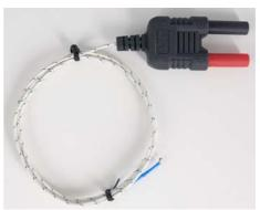
Type K thermocouple with banana plugs
